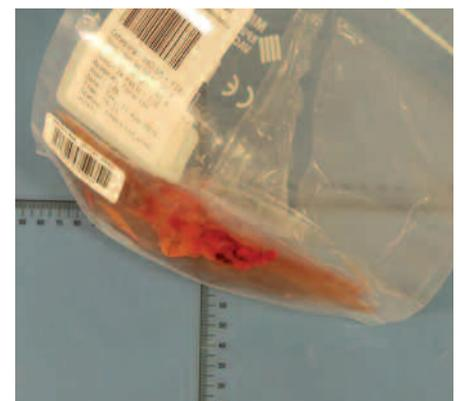
‘The bags are heat-sealed under pressure to reduce the volume and thus the space taken by the specimens’
